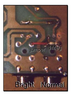
Figure 2. Main board: input jacks
