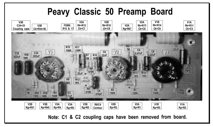
Figure 5. Component side of preamp tube board before mods begun.
