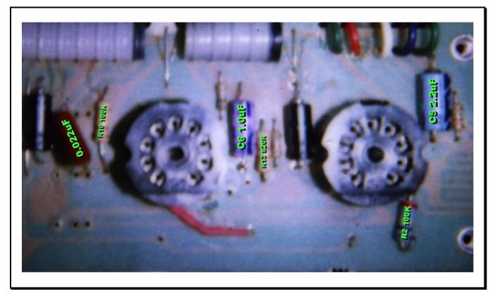
Figure 6. Component side of preamp tube board after mods completed.
